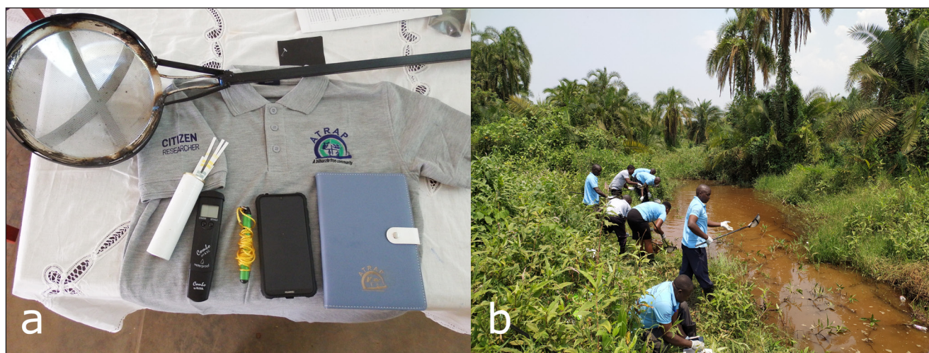
Figure 2 (a) Overview of the equipment provided to the citizen scientists: fine-meshed scoop net, ATRAP project t-shirt, water chemistry test strips, stream thermometer, smartphone, diary and Hanna Instruments pocket tester. Latex gloves, rubber boots and the laminated sheet of millimetre paper are not shown in the photograph. (b) In-field sampling exercise during the two-day training course for the citizen scientists in Kagadi.
