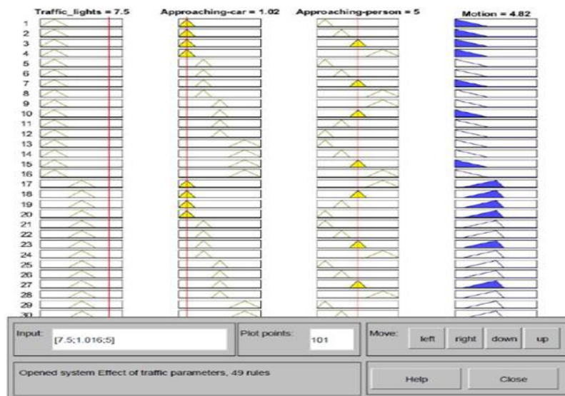
Fig. 14. Traffic light = green, Approaching car = left-lane, Approaching person = right-lane, Motion = 4.82.
