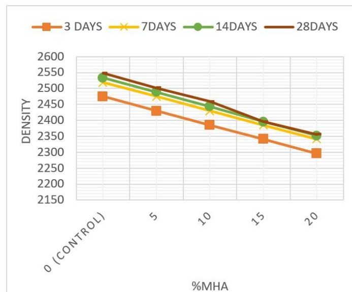
Figure 5. Line graph of density vs. MHA replacement (1:2:4 Mix).
