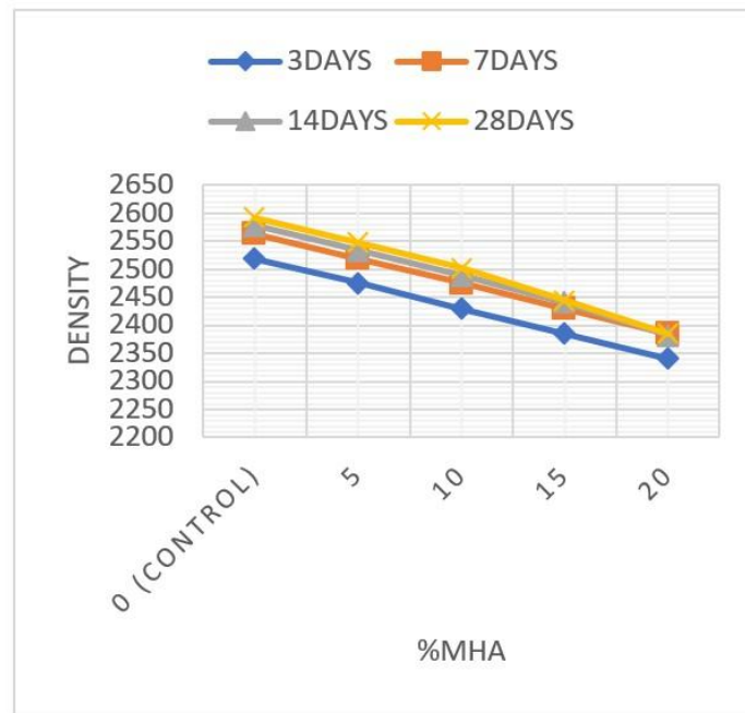
Figure 6. Line graph of density vs. MHA replacement (1:1.5:3).
